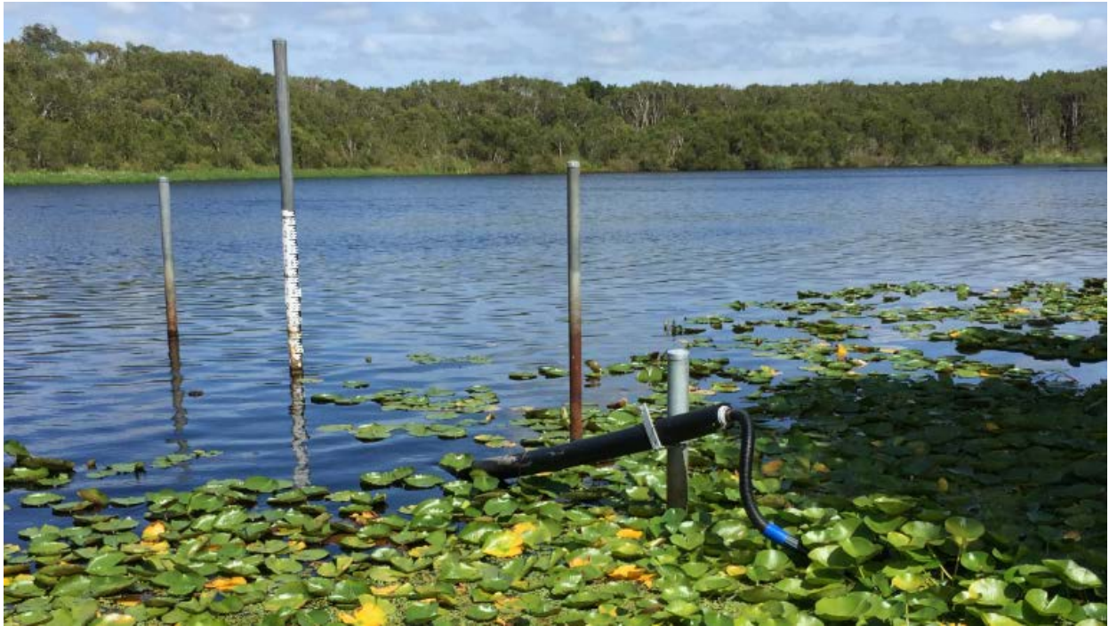
Plate 2: Water level logger deployed at northern end of Lake Ainsworth managed by MHL/OEH
